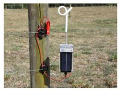
fence voltage through its clip lead, and texts the people on its list if the voltage drops below a set point. Running entirely from solar energy just like the Batt-Latch does, it carefully looks after its internal battery so the unit will always be ready for use. We'll have a demo unit on our stand at Fieldays (M30).
