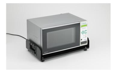
We have designed this DM% instrument, the ForageLab, to allow farmers to check progress on hay and silage before baling or wrapping, check bought-in feeds, and for agronomists to perform CWD trials quickly. The unit can also be used to check the progress of wood drying, or to dry out soil samples before analysis.
